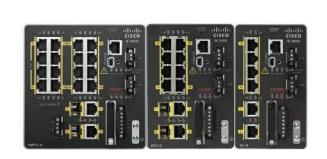
DIN-rail mounted switch with REP, IEEE 1588, Ethernet/IP, PROFINET support; 2 x GE & 4, 8, or 16 x FE ports, swappable flash memory. NAT PoE and conformal coating available.
